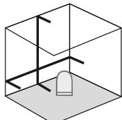
Release the transport restraint, push the slide switch (2) to the right. The laser lines can be switched individually with the selection button.
