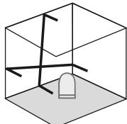
Do not release transport restraint, push slide switch (2) to the left. Sloping planes can now be measured. This mode cannot be used to perform horizontal or vertical levelling as the laser lines are no longer aligned automatically. The laser lines flash green.
